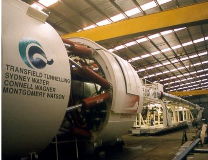
TERRATEC's Double Shield Hard Rock TBM
